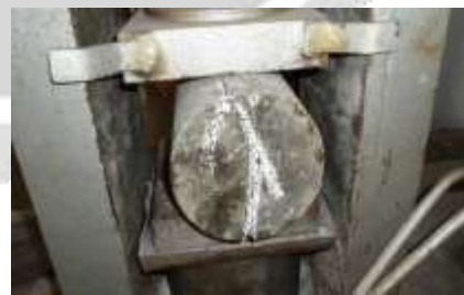
Fig 7 Failure mode of Cylinder
