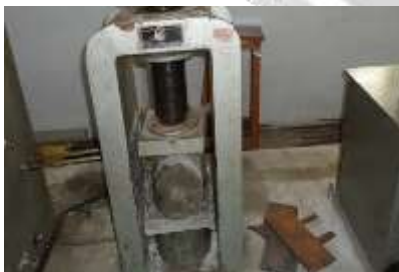
Fig 6 Test setup for Split Tensile Strength of Cylinder
