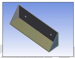
Fig.2.Steel AC mounting bracket
