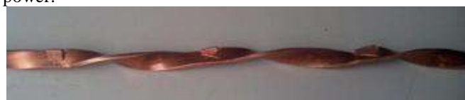
Figure-6: Square jagged copper twisted tape insert (twist ratio, y/w=7)
