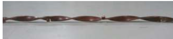
Figure-8: Square jagged copper twisted tape insert (twist ratio, y/w=4 )
