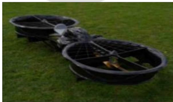
Fig. 1: Bi copter Hover bike prototype
