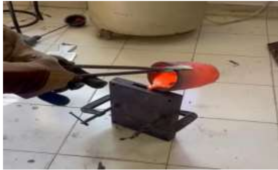
Fig.10 Pouring of mixture in the mold
