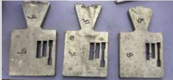
Fig.12 Material cutting process
