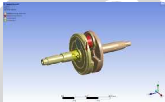
Fig -5 Applying thermal Loads and Supports
