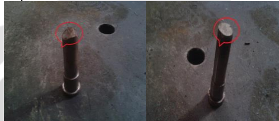
Figure 2.1: Failure of Punches
