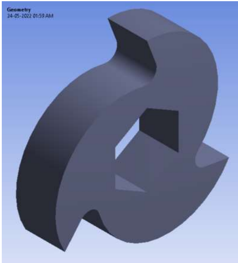
Figure 6.11 redesigned part Weight of the geometry after Topology optimization at 100 MPa Stress Retention
