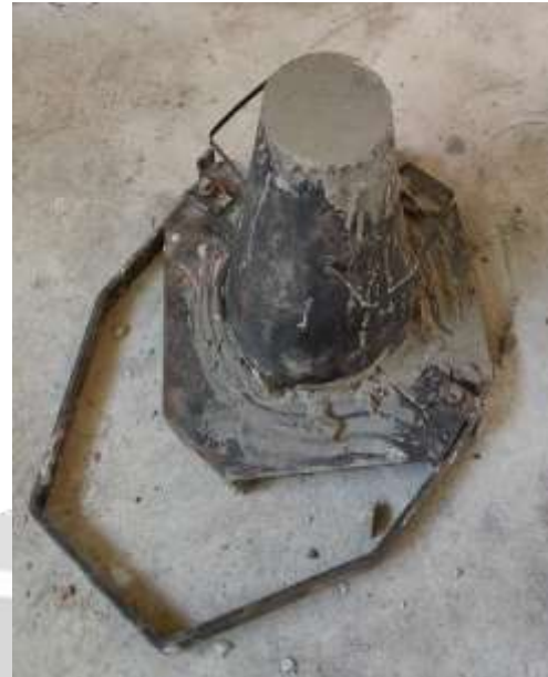
Fig-2: slump test
