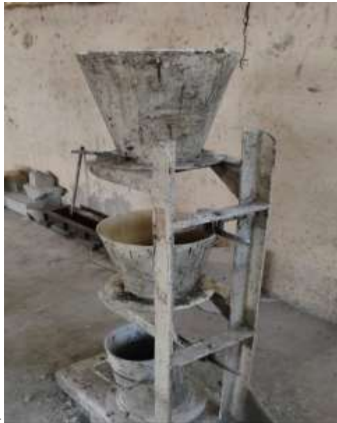
Fig-1: compaction factor test
