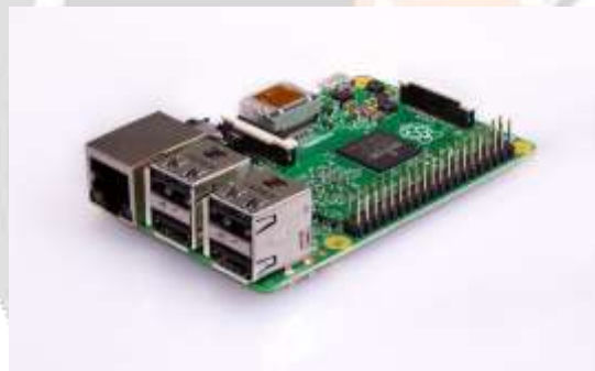
Fig 4: Raspberry Pi : A Single board computer used for purpose of experimentation for this project
