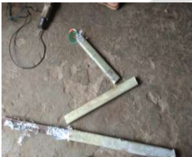
Fig-1.1.5: Rectangular cross section glass fiber shaft after detaching
