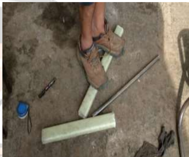
Fig-1.1.6: High strength glass fiber shafted after cutting in to required lengths
