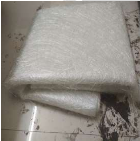
Fig-1.1.1: Glass fiber layers used
