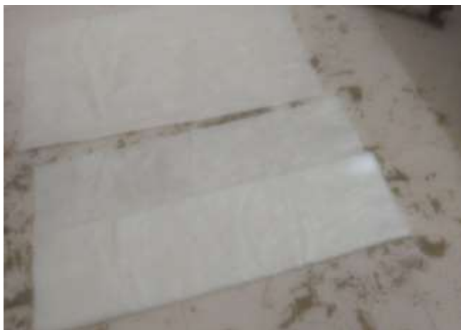
Fig-1.1.3: Layers used to form rectangular cross section glass fiber shaft
