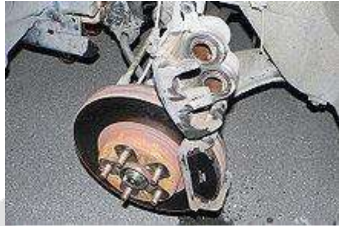
Fig 2: Disc brake caliper (twin-pot, floating) removed from brake pad for changing pad
