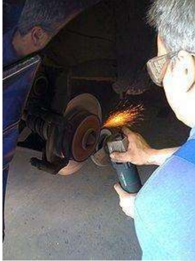
Fig 1: Disc Brake being polished after scarring occurred
