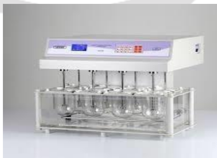
Fig N0. 7 Dissolution test apparatus
