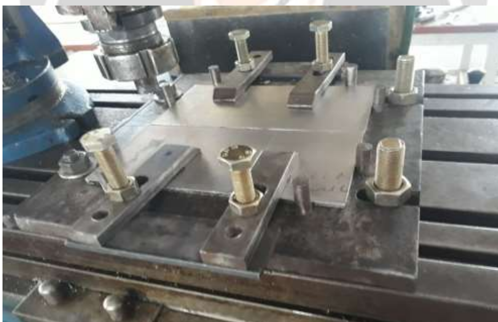
SPECIMEN FIXED IN FIXTURES
