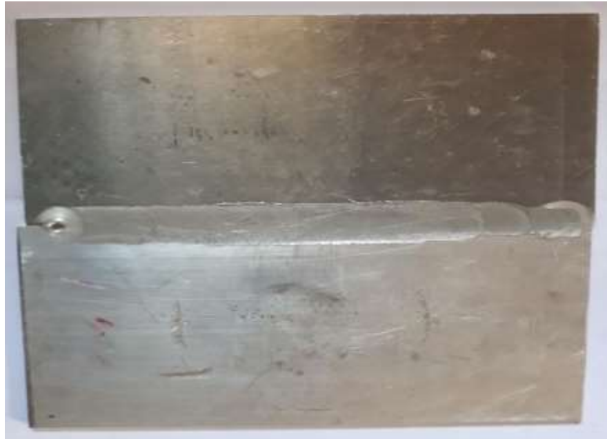
DISSIMILAR ALUMINIUM ALLOY AA6063 AND AA5052
