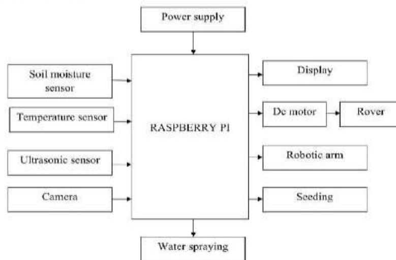
Fig.3.1 Block diagram of proposed system.
