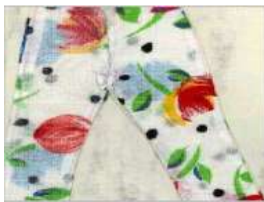
Reversed garment parts where part is sewn with the face outside opposite from specification
