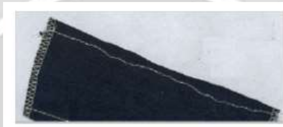
Fig No: 13 Staggered stitch is like Zig Zag Stitch
