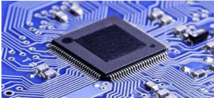
A microcontroller is a compact integrated circuit designed to govern a specific operation in an embedded system. A typical microcontroller includes a processor, memory and input/output (I/O) peripherals on a single chip.
