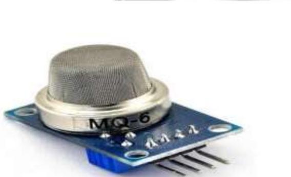
The MQ6 (LPG Gas Sensor) is a simple-to-use liquefied petroleum gas (LPG) sensor. It can be used in gas leakage detecting equipment in consumer and industry applications, this sensor is suitable for detecting LPG, iso-butane, propane, LNG. Avoid the noise of alcohol, cooking fumes and cigarette smoke.
