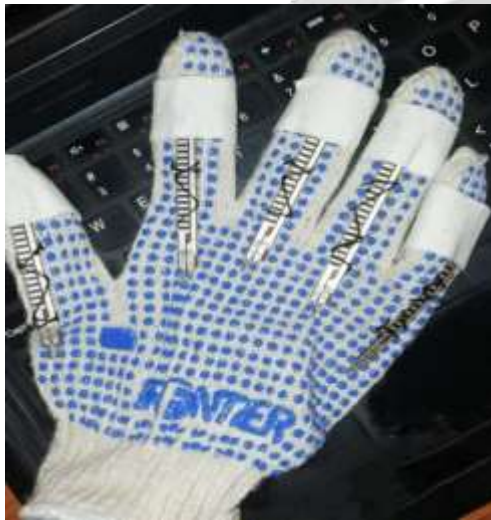
Fig -3: glove containing flux sensor
