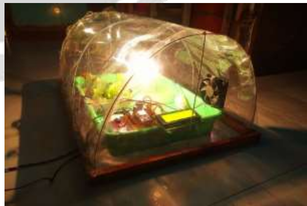
Fig -4: Implemented prototype of smart greenhouse
