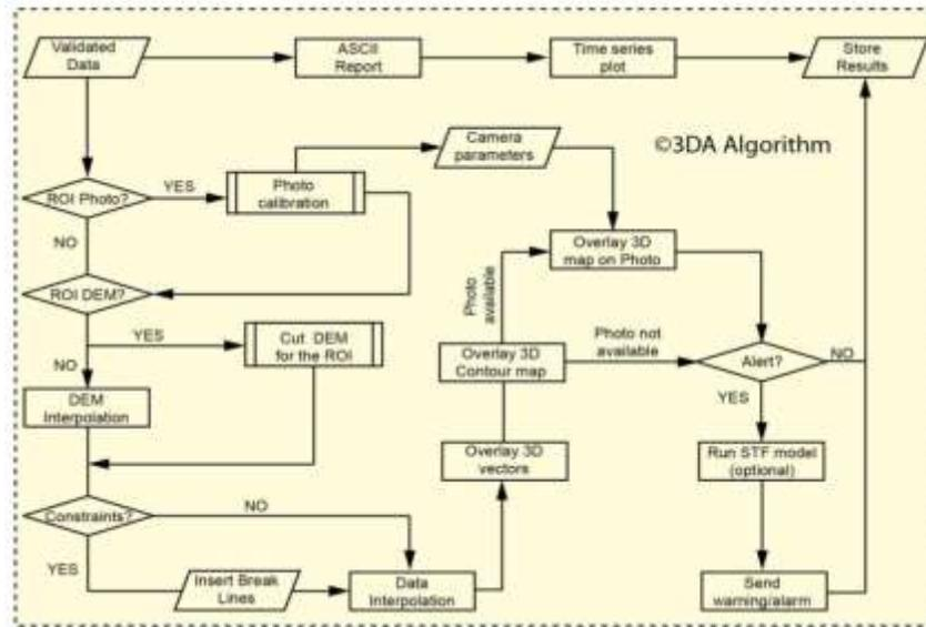
Fig. 3. Detailed flow chart as implemented in Matlab.
