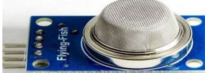
Fig-4.3: LPG Gas Sensor Module
