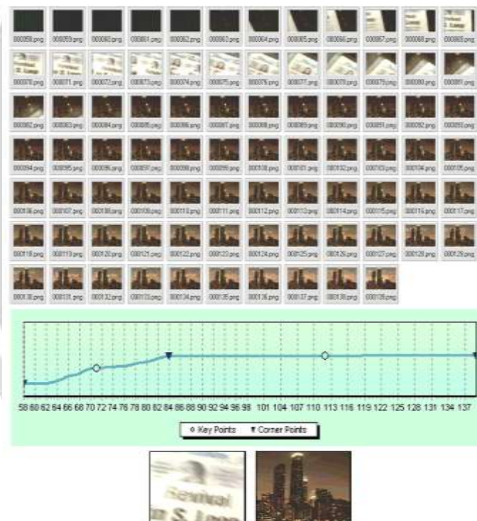
Fig. 3.4. An example of key frame selection with the proposed method. Top: the shot to analyze. Center: the corner points detected (triangles) and the key frames selected (circles). Bottom: the two key frames, number 71 and 112, extracted from the example shot are shown at the bottom.
