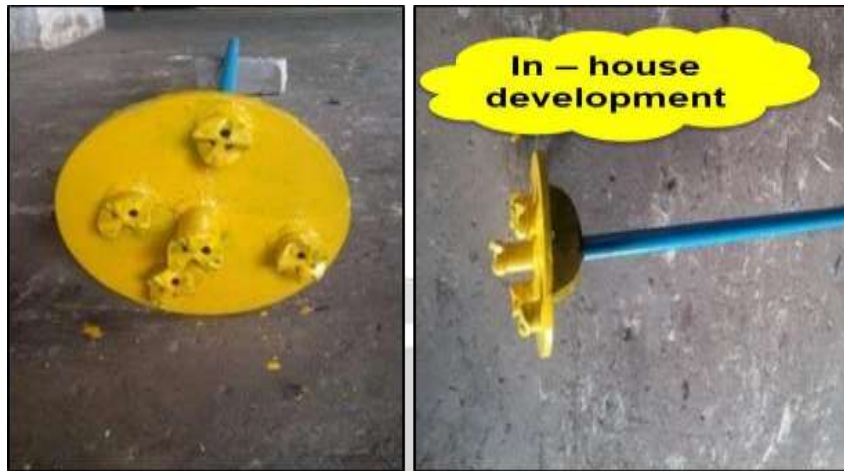
Figure 11 Elimination of hot metal exposure during tap hole cleaning
