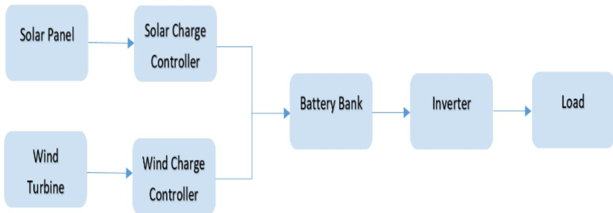
Fig -1: Solar-Wind Hybrid System
