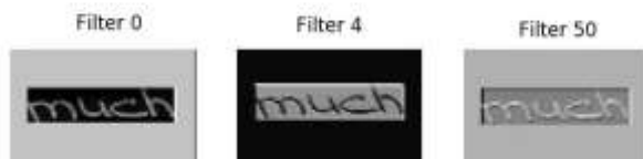
Figure 3. These are the filters from the first convolutional layer of the RESNET-18 word segmentation model with the example word "much"
