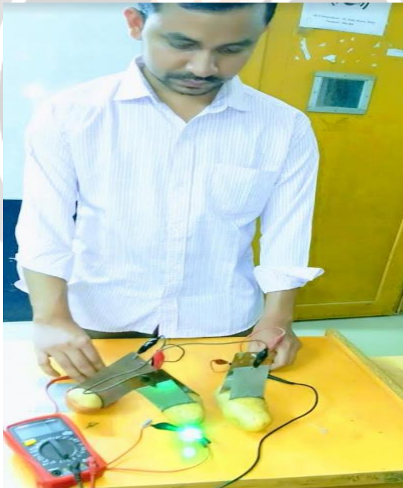
Fig.11: Experimental setup of a LED light using potato.
