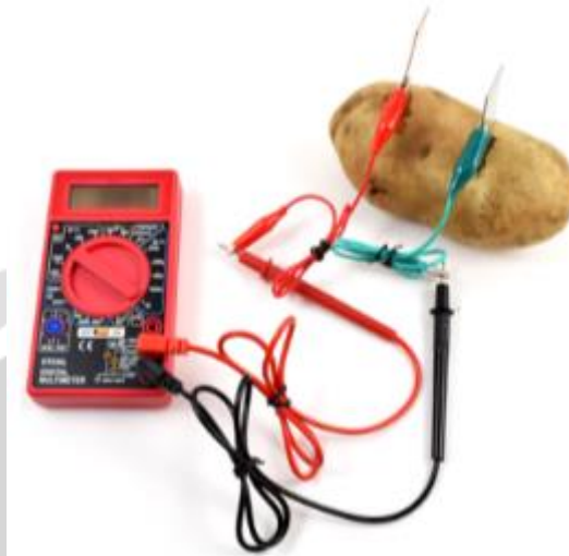
Fig. 3: Shows a multimeter set up to capture open-circuit voltage.
