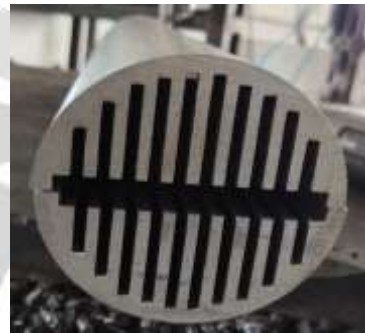
Fig 2: Alufer tube section used in test setup
