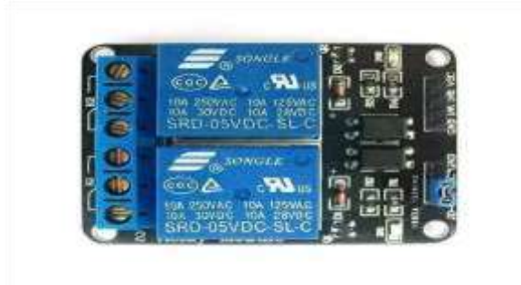
Fig 4: Relay H152S module
