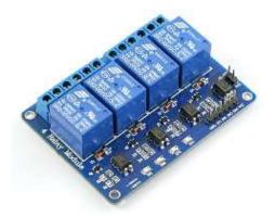
A power relay module is an electrical switch that is operated by an electromagnet. The electromagnet is activated by a separate low-power signal from a micro controller. It can be used to control high voltage high current as motor, lamps, AC load.
