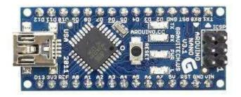
The ARDUINO Nano is small component and when using on breadboard it is user friendly .
