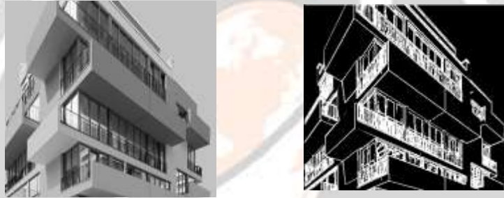
Fig -12: Results for image processing using Sobel filter
