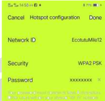
Fig.-3. SSID and password for access point to match raspberry pi 3 credentials
