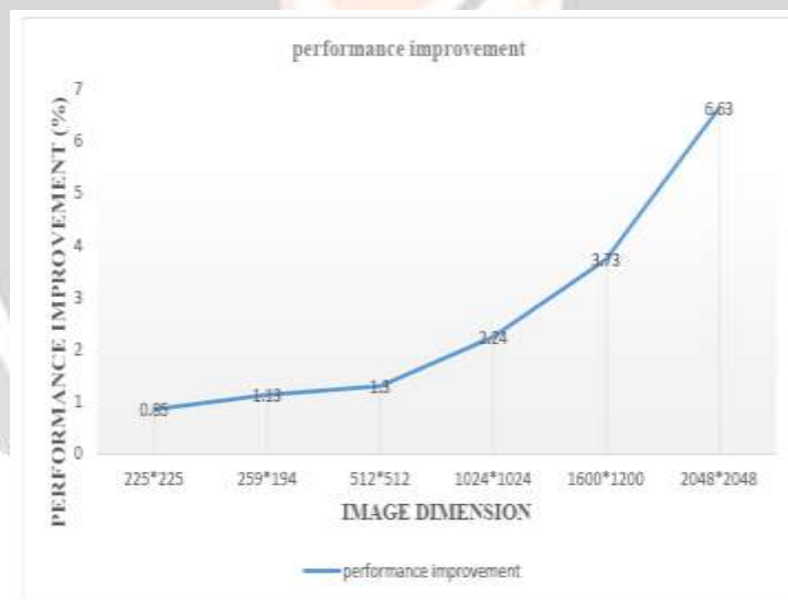
Chart -4: Performance Improvement in execution Time (%) in GPU (CUDA) compare to Integrated program execution
