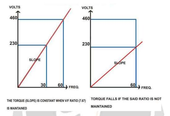
As the above theory should have helped you understand a frequency inverter, the next page will explain the operating principle of a frequency inverter.
