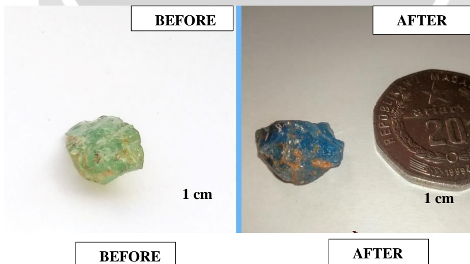
Fig-5 Sample B002 had a yellowish-green hue before treatment, and after heating to 400°C it took on a blue hue
