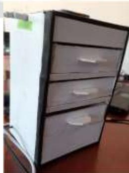
It is having three compartments to store the medicines, and compartments are driven by the servo motors. This box is compact, accessible, handy, and easy to use.
