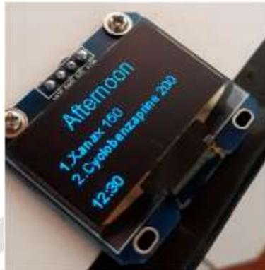
This module display is mono colored and is triggered by the ESP32, display will perpetually be on. It is helpful in displaying the medicine's names and their timings that patient can view and consider it accordingly.
