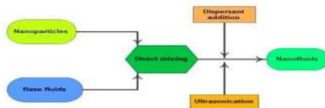
Fig -2 Two-step preparation processes of nanofluids.
