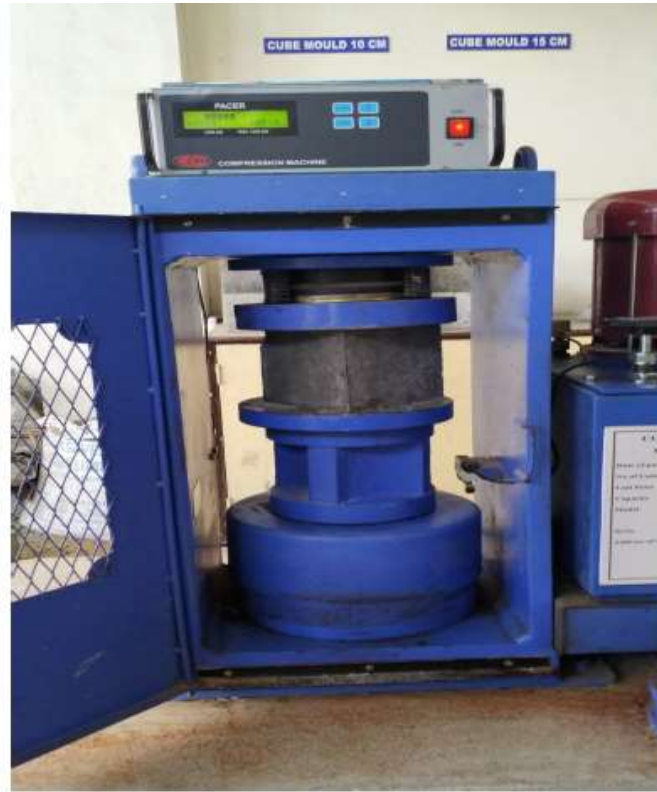
Fig -1 Specimen for Compressive Strength
