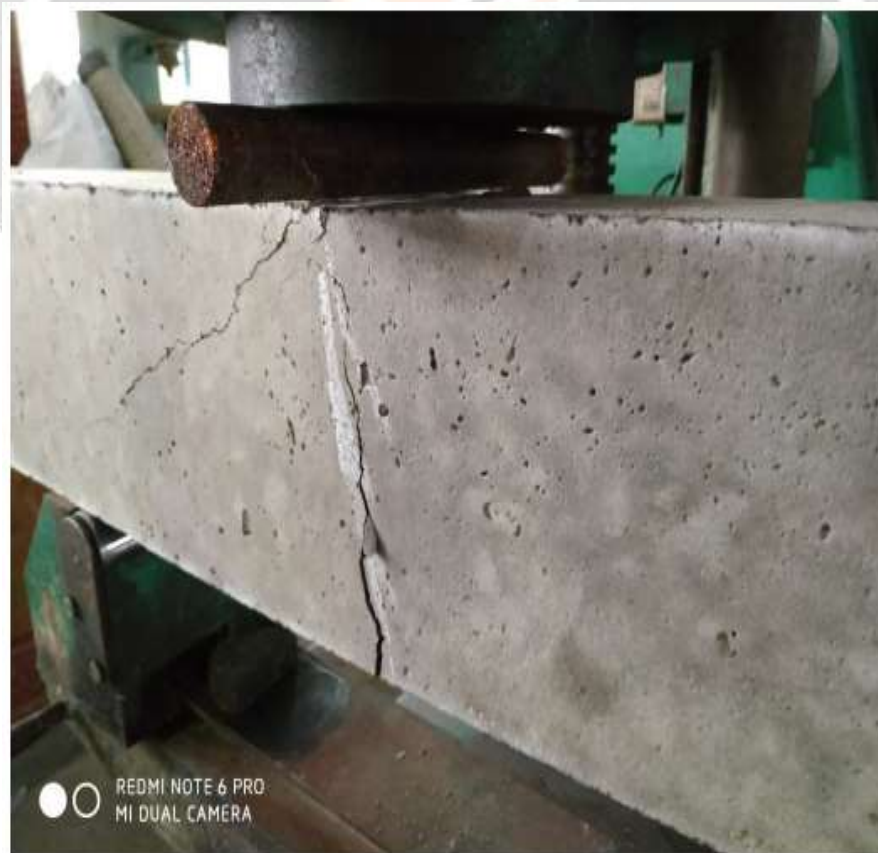
Fig -3 Cracks obtained while applying load at mid span
