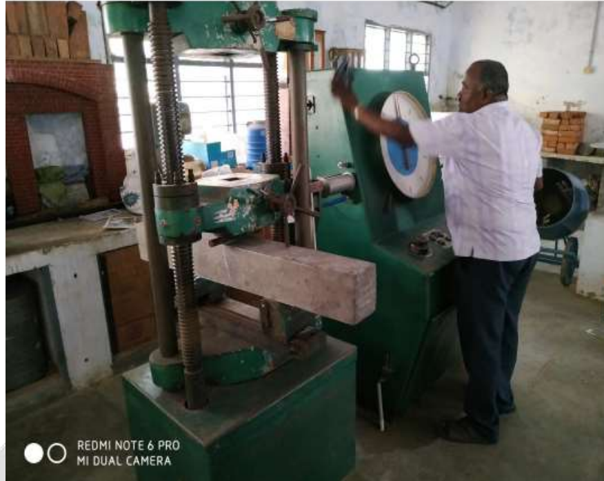
Fig -2 Beams testing in universal testing machine
