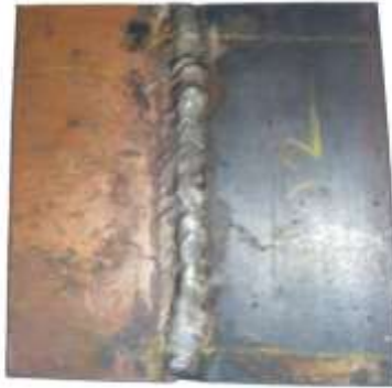
Fig -7: Cu and MS TIG Welding Using Copper Filler Rod:
