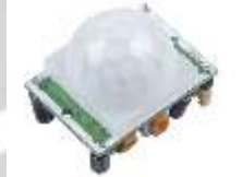
Fig 4.2. PIR Motion sensor.
