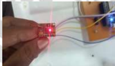
Fig -5 Heartbeat and Oxymeter Sensor
