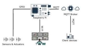
Raspberry pi use as an interface between devices and web dashboard through wireless connection. In this proposed system we used temperature and humidity sensor, LPG and smoke detection
