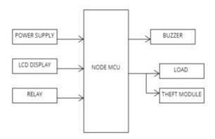
The device is characterized by easy access to the data and therefore the combination of a smart meter and digital communication capability allows local and remote access. In this way, it is possible to manage the power consumption by the electrical appliances and also check the amount of power consumed by our appliances in terms of money. The Wi-Fi unit performs the IoT operation by sending energy meter data to the cloud which may be accessed and displayed on an LCD screen.
