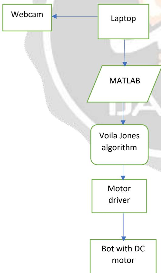
For simplicity, we have attached an IR web camera onto the handle part of the Wheelchair that is used to detect the eye motion. Then we have designed an algorithm to track the iris part of the eye using centroid calculation
