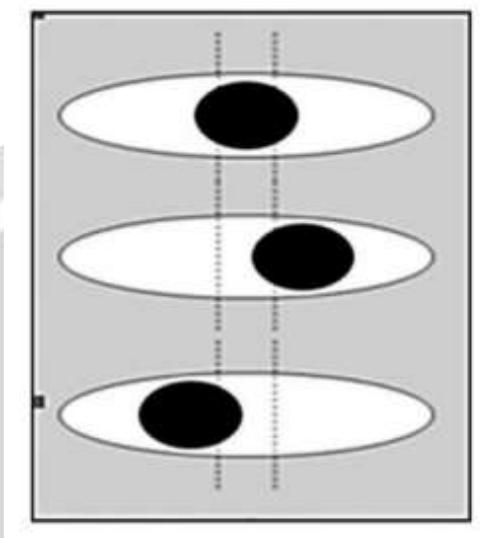
Image of the pupil is extracted and an arbitrary distance is calculated from the centre of the pupil to the corner of the eye. This distance is used to decide whether to turn the wheel chair left, right or keep moving forward.
