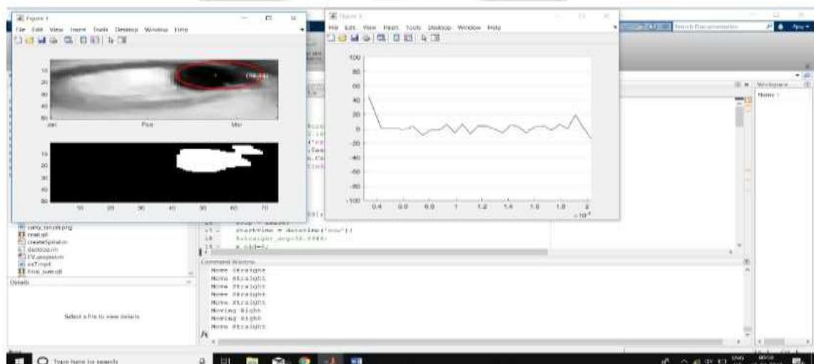
The above result is obtained for the right motion tracking of the iris. The left wheel of the bot stops moving for a small moment and as a result, the bot turns towards to the right. When the iris is detected in the left position, the right wheel of the bot stops for a second and then starts spinning again as a result the bot turns left. As long as the iris is detected in the centre position, the bot will keep on moving forward.
