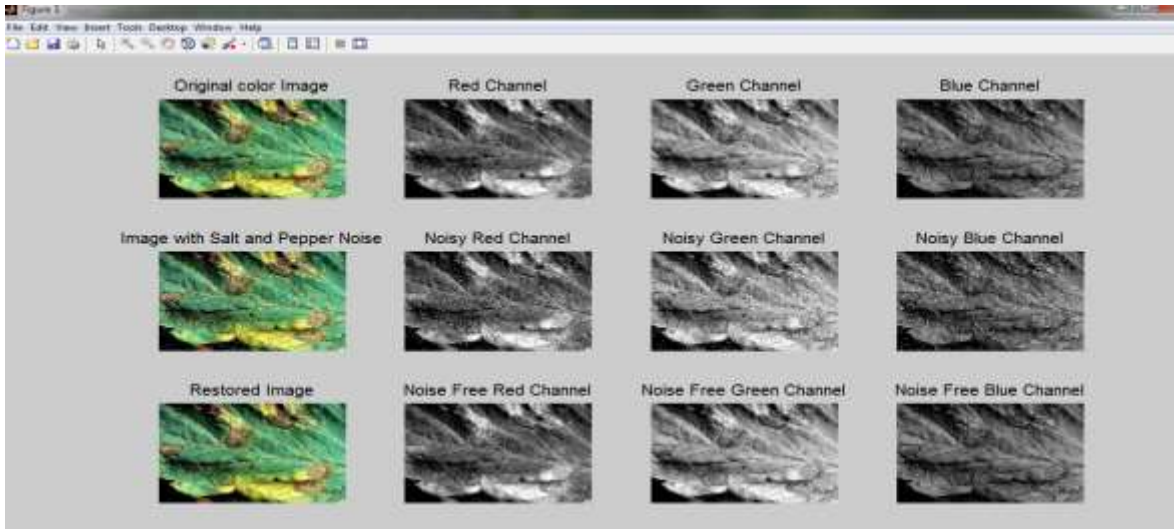
Fig 4.3: Filter results with Red, Green and Blue Channel color transformation structure from RGB
