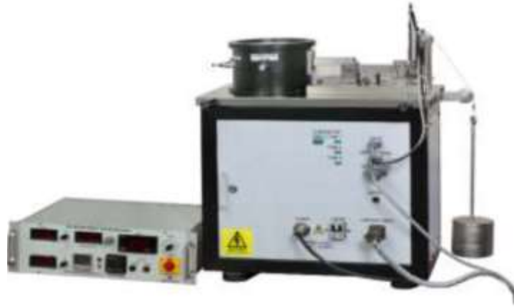
Fig -5: Pin on disc wear test apparatus
