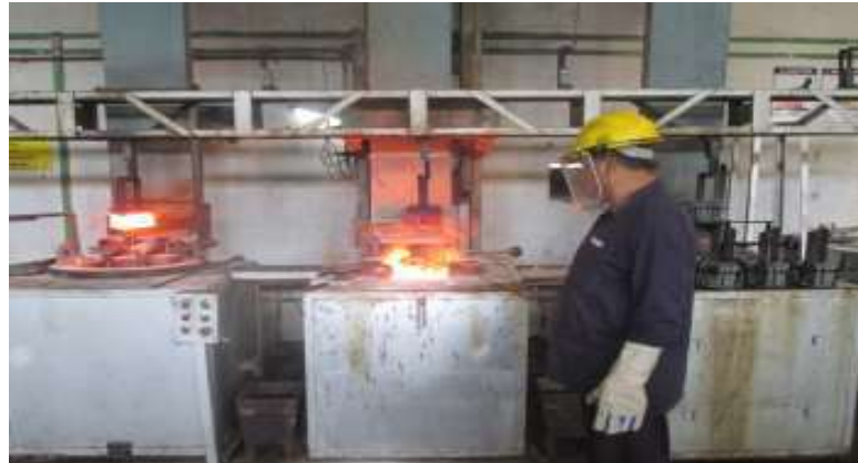
Fig -2 : Auto Hardening Setup Installed at JKFIL, Chiplun
