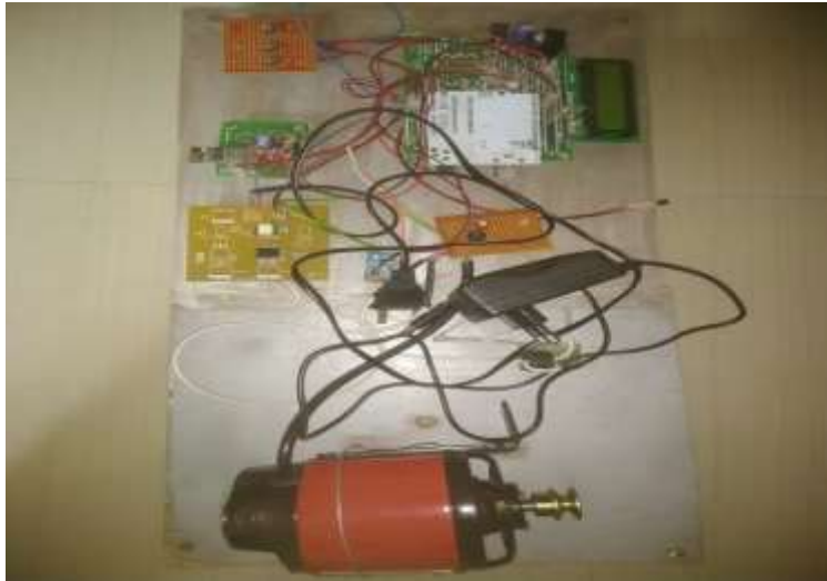
Fig. 4 A laboratory prototype of IoT based bidirectional speed of single-phase induction motor
