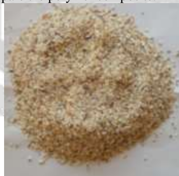
Figure 1.1: Sieve analysed seashell grain particles of 850\mu\text{m}
