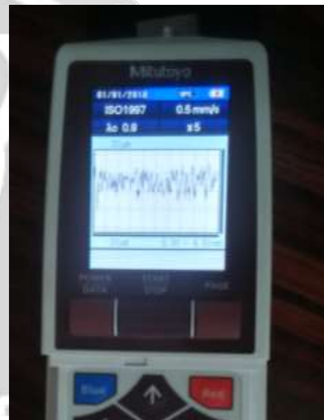
Figure 5: Surface Roughness graph
