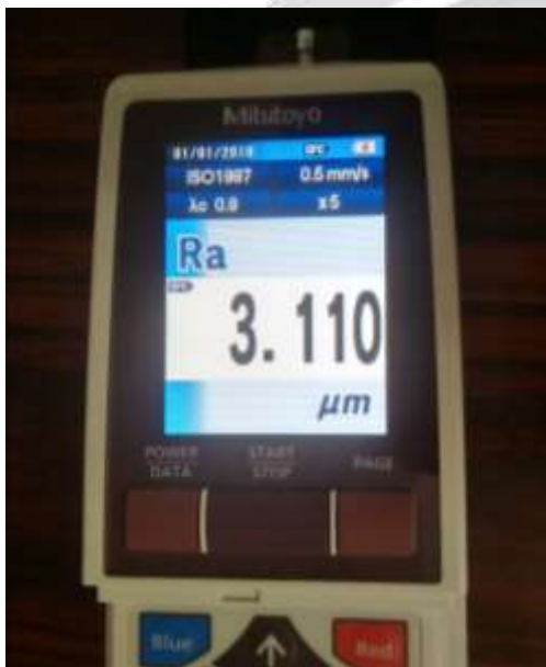
Figure 4: Measurement of Surface roughness of cut profiles
