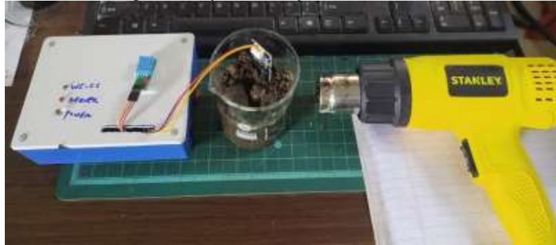
Fig 5.12 : Iot data logger with external variable Temperature source by hot air gun
