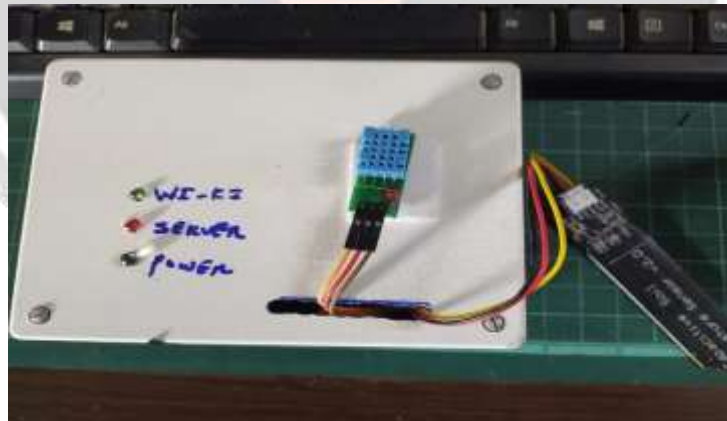
Fig 4.2: Iot Data Logger with DHT11 and Soil Moisture Level sensor
