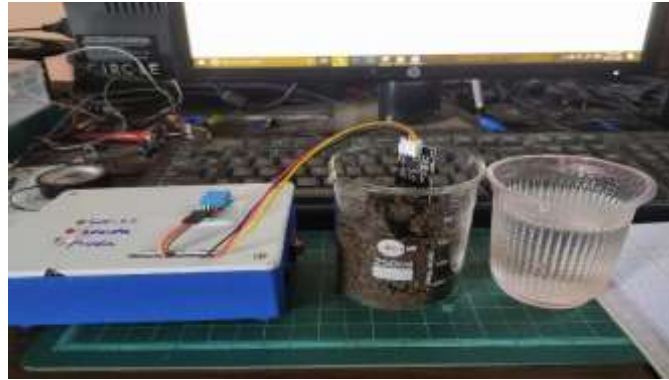
Fig 1.3 : Iot Data Logger with dht11 and soil moisture level sensor in real time testing mode
