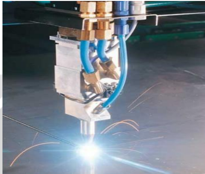
Figure 1 Laser Welding Process
